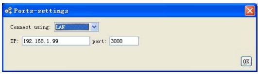
Figure 6-5: Set the network parameters of the ultrawave software
