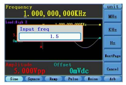
Figure 5-2: Set the frequency using number keys
