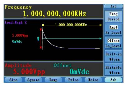
Figure 5-12: The Exponential Fall Waveform
