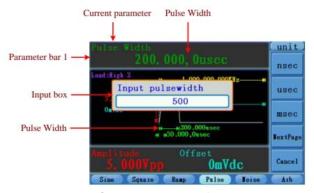
Figure 5-8: Set the Pulse Width of Pulse signal
