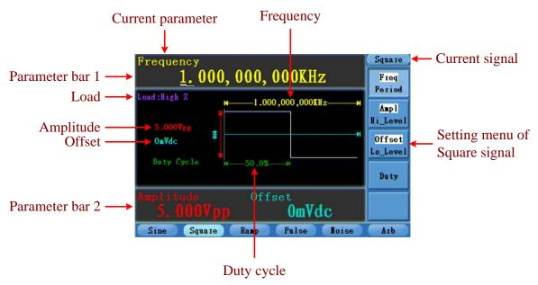
Figure 5-3: The User Interface of Square Signal
