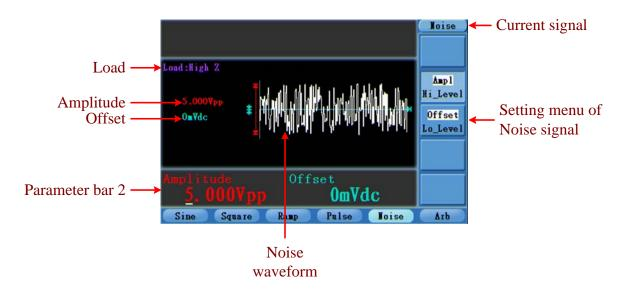
Figure 5-10: The User Interface of Noise Signal
