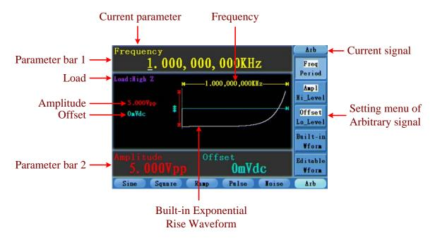
Figure 5-11: The User Interface of Arbitrary Signal
