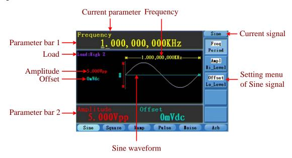
Figure 5-1: The User Interface of Sine Signal
