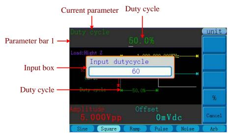
Figure 5-4: Set the Duty cycle of Square signal
