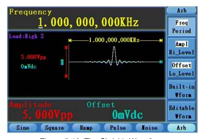
Figure 5-13: The Sin(x)/x Waveform
