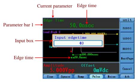
Figure 5-9: Set the Edge Time of Pulse signal
