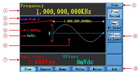
Figure 4-3 User interface (take Sine for instance)
