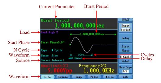
Figure 5-20: The User Interface of N-Cycle Burst
