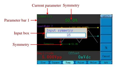
Figure 5-6: Set the symmetry of Ramp signal
