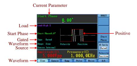
Figure 5-21: The User Interface of Gated Burst
