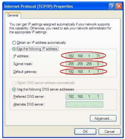
Figure 6-4: Set the network parameters of the computer
