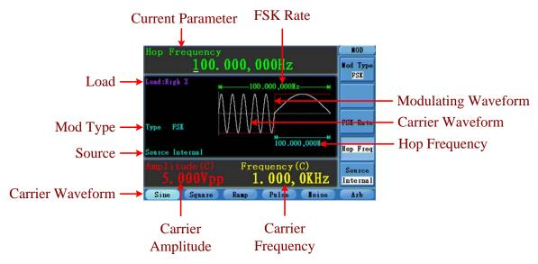
Figure 5-17: The User Interface of FSK
