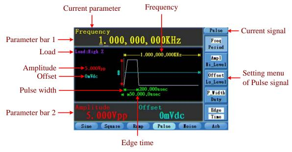
Figure 5-7: The User Interface of Pulse Signal
