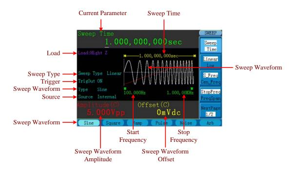
Figure 5-19: The User Interface of Sweep Mode
