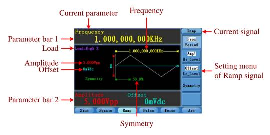
Figure 5-5: The User Interface of Ramp Signal
