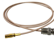
Thermal vacuum (TVAC) trigger cable, BNC male to SMB female, 50 \Omega , 1.5 m (Quantity: 2) (for Option TVA)
