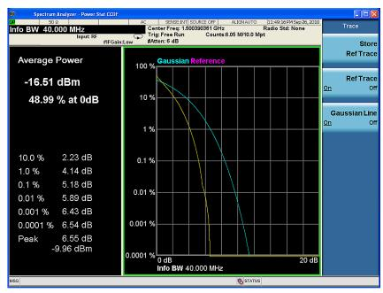
40 MHz bandwidth CCDF measurement (Option B40 required)
