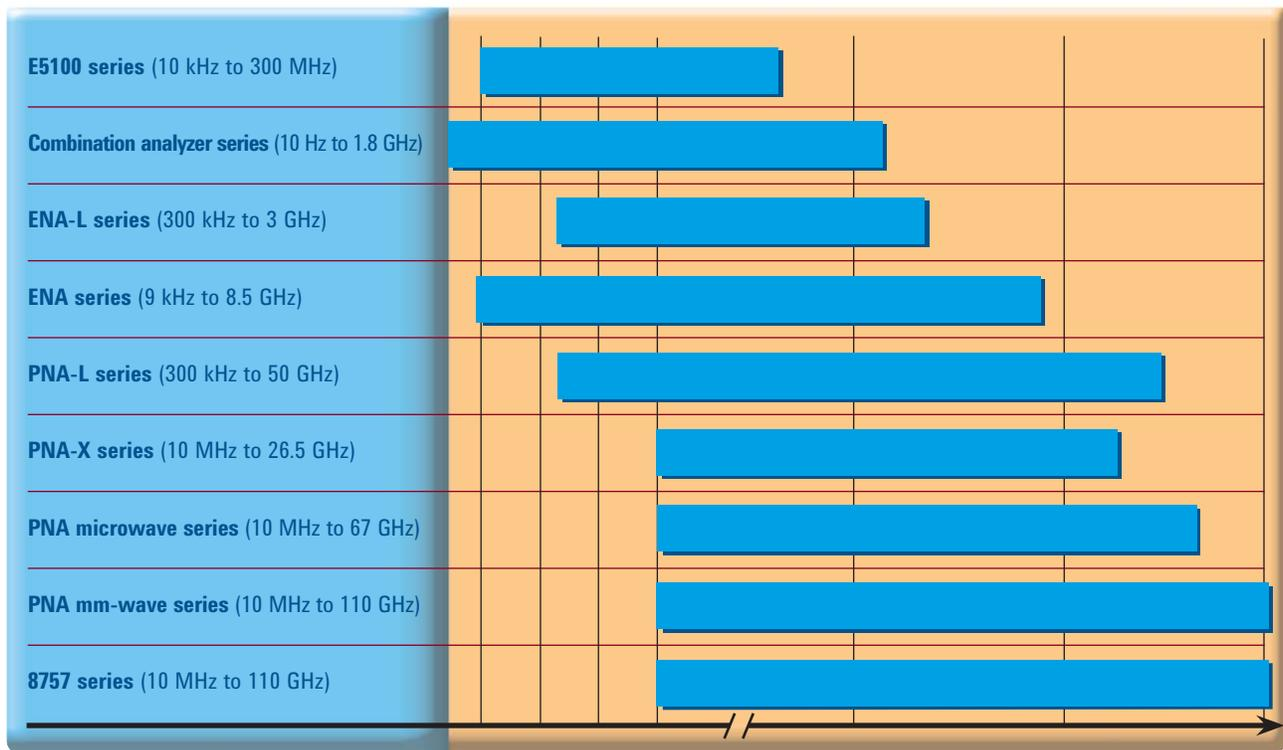
Frequency coverage for Agilent network analyzers
